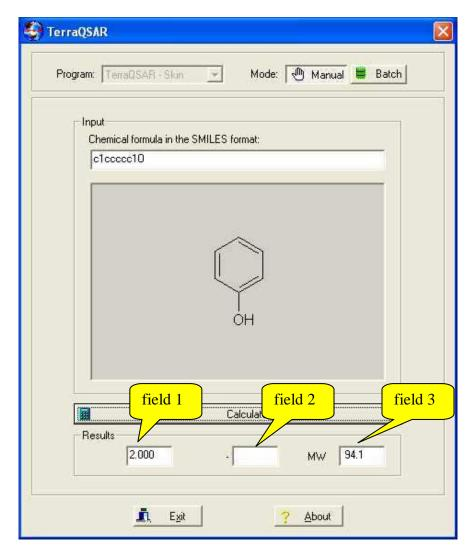
**Fig. 4**. Result of the execution of "Calculate". The fields show the following values: Field 1 (without label) is the skin irritation potential as described above. Field 2 is unused, and field 3 shows the molecular weight of the compound. Example shows the computed value for phenol (2.00), indicating a strong dermal irritant.
